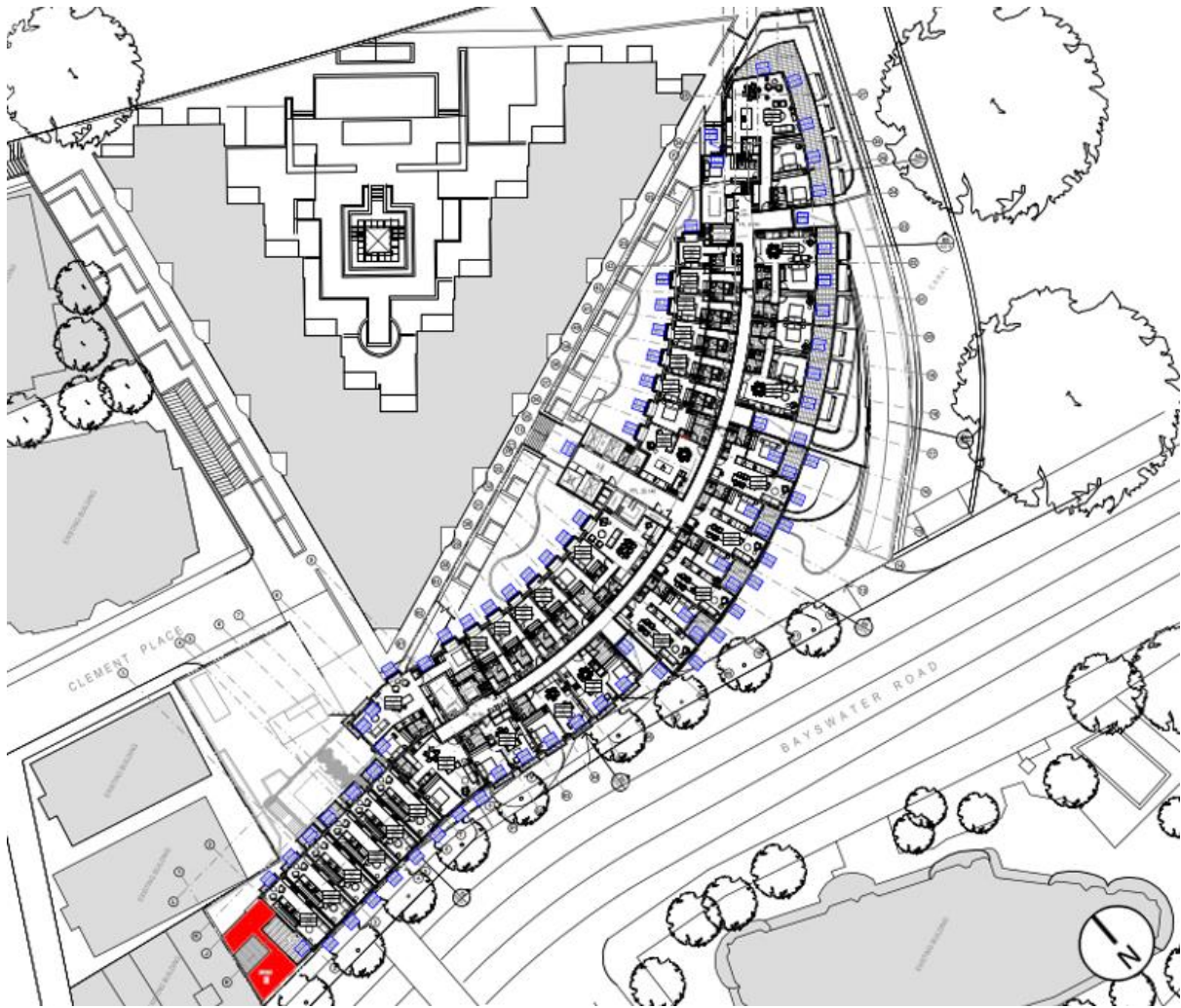
Figure 17: Proposed Level 5 (with proposed roof modification from synthetic turf to river pebbles shown in red)
