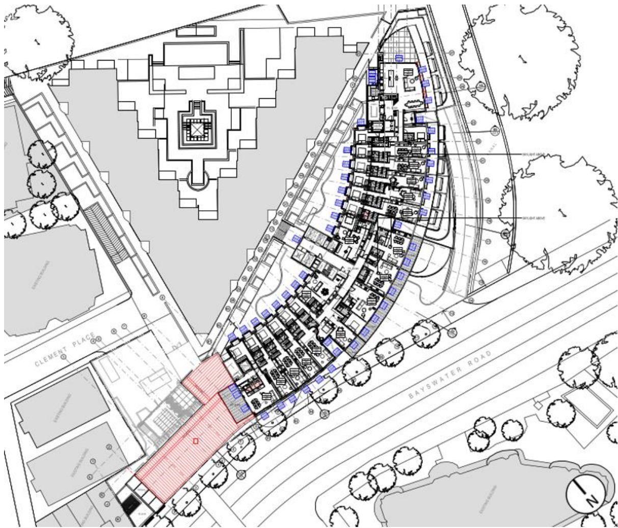
Figure 18: Proposed Level 6 (with proposed roof modification from synthetic turf to metal sheeting shown in red)
